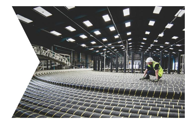
JDR designs, manufactures, delivers, and supports subsea production umbilicals, subsea power cables and Intervention Work Over Control Systems (IWOCS) for installation at everincreasing depths.
